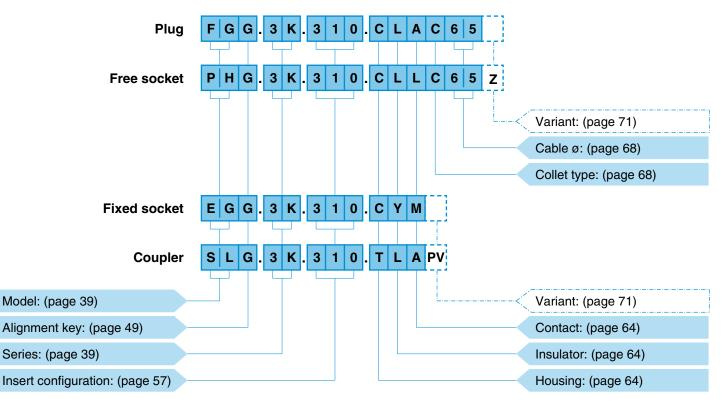
**FGG.3K.310.CLAC65** = straight plug with key (G) and cable collet, 3K series, multipole type with 10 contacts, outer shell in chrome-plated brass, PEEK insulator, male solder contacts, C type collet for 6.5 mm diameter cable.
