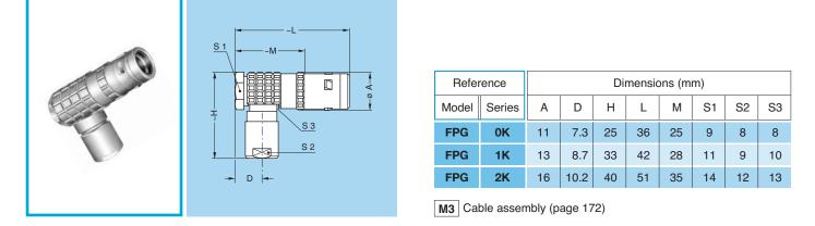
FHG Elbow (90°) plug, key (G) or keys (A to F, L and R), cable collet
