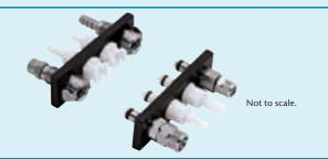
**72** Multi-Mount: Connects three to five lines at once; keyed to prevent mismatched connections. Material: Acetal, chrome-plated brass Tubing ID Sizes: 1/8" to 3/8" (3.2mm to 9.5mm)
