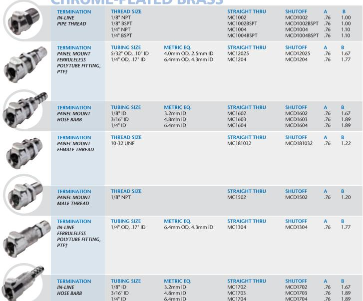
All measurements are in inches (millimeters) unless otherwise noted. Tubing must meet stated inside and outside diameters. †NOTE: Colder's Ferruleless PTF (polytube fitting) terminations do not require ferrules to achieve a secure connection and are therefore easier to use and reuse. PTF fittings are designed for semi-rigid tubing, i.e., polyethylene, nylon, polyurethane, etc. NOTE: Elbow configurations are available. Contact Colder for more information.
