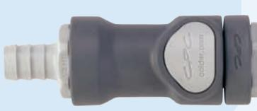
**54** NS6: Durable, yet lightweight construction that features non-spill valves and is compatible with many chemicals. Material: Glass-filled polypropylene Tubing ID Sizes: 3/8" to 1/2" (9.5mm to 12.7mm)
