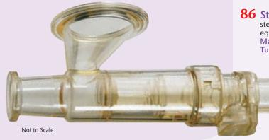
**86** Steam-Thru® Connections: Allow quick and easy sterile connection between biopharmaceutical processing equipment and disposable bag and tube assemblies. Material: Medical-grade polysulfone **Tubing ID Sizes:** 3/8" and 1/2" (9.5mm and 12.7mm)
