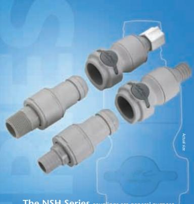
The NSH Series couplings are general purpose versions of our pressure-balanced, non-spill, ChemQuik® CQG06 couplings. Molded polypropylene, EPDM seals and a 100% springless and metal-free flow path provide broad chemical resistance and exceptionally high flow capacity, allowing instant disconnects (and reconnects), even under pressure. Their non-spill design virtually eliminates spills, minimizes downtime and enhances operator safety in a very low cost package.
