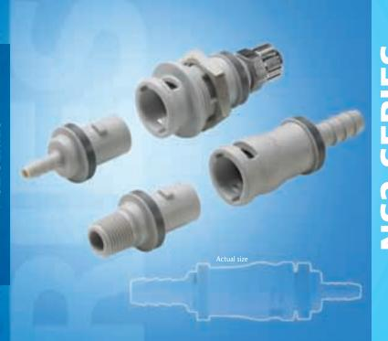
The NS2 Series couplings were built on the company's proven platform of non-spill valves designed to provide fast, safe and virtually leak-free fluid line connections. The NS2 offers an easy, twist-to-connect coupling with an integrated locking mechanism and double-sided non-spill shutoff valves. The NS2 is also chemically resistant making it ideal for a diverse range of applications.
