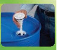
3 Turn shipping plug counter-clockwise to remove. (Use a large, flat blade or #4 Phillips screwdriver.)
